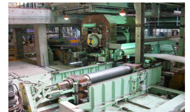
张家港浦项不锈钢四辊平整机 Stainless steel four-roll SPM of Zhangjiagang Pohang Stainless Steel Co., Ltd.
