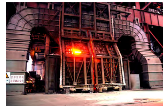
马钢四钢轧总厂转炉工程-国内最大转炉 BOF project of NO.4 Steel Making and Rolling General of Masteel--The largest BOF in China
